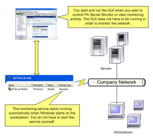
The service is the part of the product that performs the monitoring of the network. The service is set up so that it runs automatically when Windows starts. The Console does not need to be running in order for monitoring to take place.
