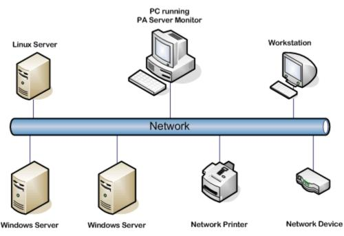
The PA Server Monitor product is composed of two parts: a graphical user interface that we call the Console, and a background process called the monitoring service. You see the Console when you launch PA Server Monitor from the desktop. The service is invisible and has no user interface of its own.
